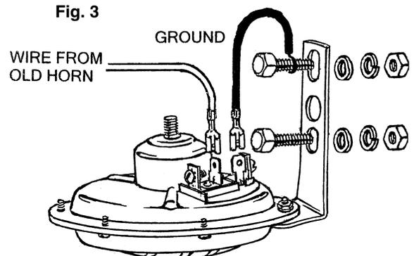
4. The other horn terminal is connected to ground using any of the following locations; under the horn's mounting bolt if mounted on a metal body surface, under any clean metal body bolt or the (-) negative post of the battery. Always make sure the metal ground surface is free of paint, rust and oxidation.
