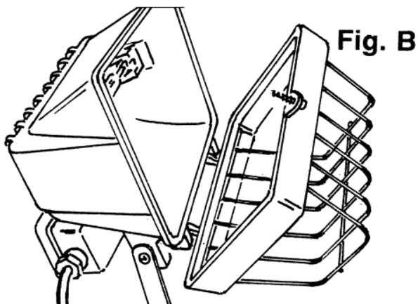
7. The lens cover will now open. To remove the old bulb, simply push the bulb gently to the right until the left hand side of the bulb slides out of the electrical socket.
