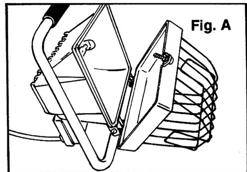
5. To remove the old bulb, simply push the bulb gently to the right until the left hand side of the bulb slides out of the electrical socket.
