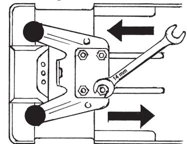
8. Remove the tension adjustment bolts from brackets located on the bottom of the light bar. See fig. 4.
