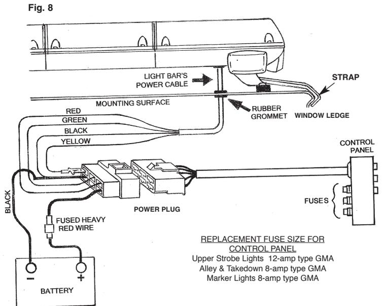
22. Route the heavy gauge RED & BLACK wires to the vehicles battery. If the power wires pass through any drilled holes or firewall, always use a rubber grommet to protect the vehicle.
