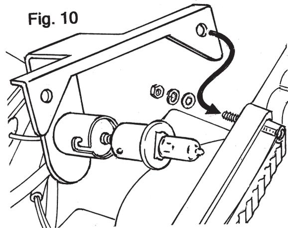
30. To remove bulb simply press inward and turn counter clockwise. The bulb should easily be able to be removed from the socket. Dispose of the bad bulb out of reach of children and in an environmentally safe manner. See fig. 10.
