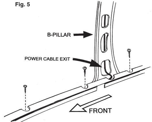
16. Make sure the power cable has been completely pulled into the vehicle, use silicon or similar waterproof material around the grommet and power cable to ensure a waterproof installation.
