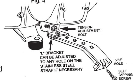
11. Tighten the two-(2) tension adjustment bolts evenly. While tightening the bolts make sure the light bar remains in the desired mounting position on the roof. Torque bolts to 10-12 ft-lbs. Failure to properly tighten the tension adjustment bolts and straps could result in damage to the vehicle and/or injury to driver or others.
