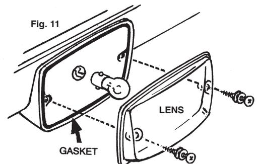
37. To remove bulb simply press inward and turn counter clockwise. The bulb should easily be able to be removed from the socket. Dispose the bad bulb out of reach of children and in an environmentally safe manner.
