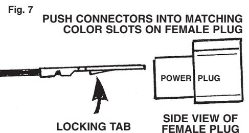
**NOTE:** The plug's middle position between the heavy gauge red and black wire is not used for this model light and should remain empty.
