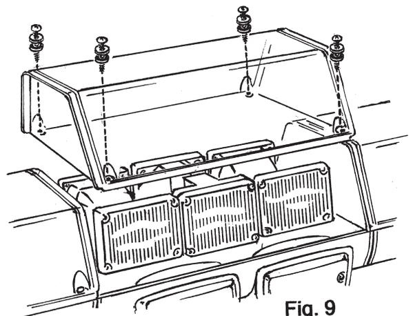
28. Replacement bulb type: use only halogen 796/35watt halogen, 12 volt. Current draw: 2.73 amps.
