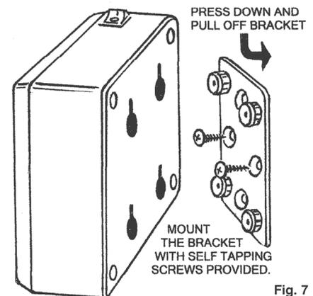
17B. **SCREW METHOD:** Remove the mounting bracket from the back of the switch controller by gently pushing downward on the bracket while pulling from the switch controller. Using the mounting bracket as a template, mark the two screw hole locations and drill to size. 7/64". See fig. 7
