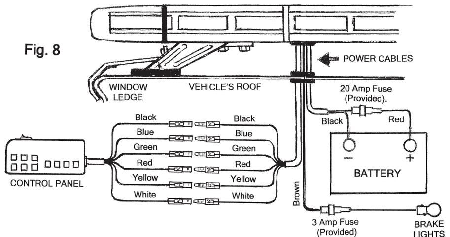
23. **RED WIRE:** Connect to positive (+) 12-volts such as the fuse block, accessory power source in the dashboard area or the positive (+) battery post. Always use the provided 10-amp inline fuse. Make sure the connection is at a location free from corrosion or oxidation.
