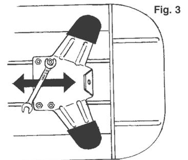
8. Remove the tension adjustment bolts from brackets located on the bottom of the light bar. See fig. 4.
