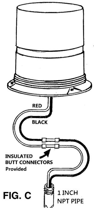
**IMPORTANT:** If the extension wires are not RED & BLACK note the colors that are connected to the light so to ensure correct polarity when wiring to the power source.
