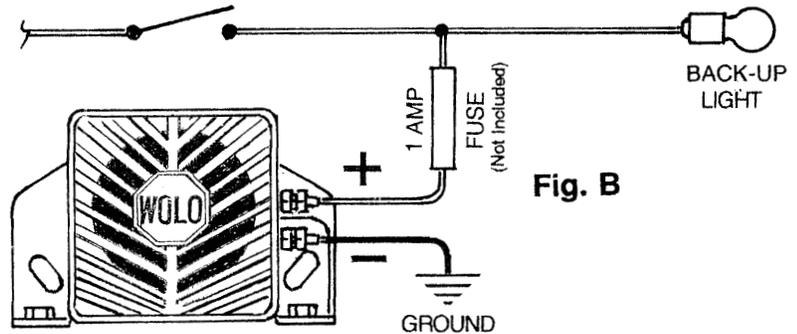
alarm must have a good connection to both power and ground to work reliably. Use 18-gauge wire (minimum) to lengthen wire leads if required. Make sure that all wires are secured and inspect to insure that they will not interfere with vehicles operation. Always make sure that any wiring is in accordance with the vehicle manufacturer's recommendations.
